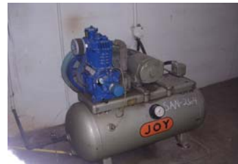
SAN-264 Compressor Unit
